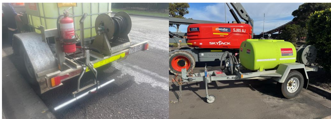
Figure 19: Concept trailer mounted road pressure washer and “Kapture” wetting agent trial water cart.
