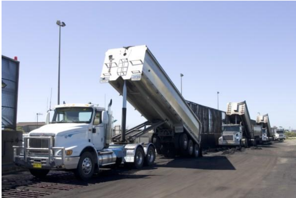
Coal is tipped into the under road hopper for conveyor transportation to the stockyards. Wind barriers assist dust control.
