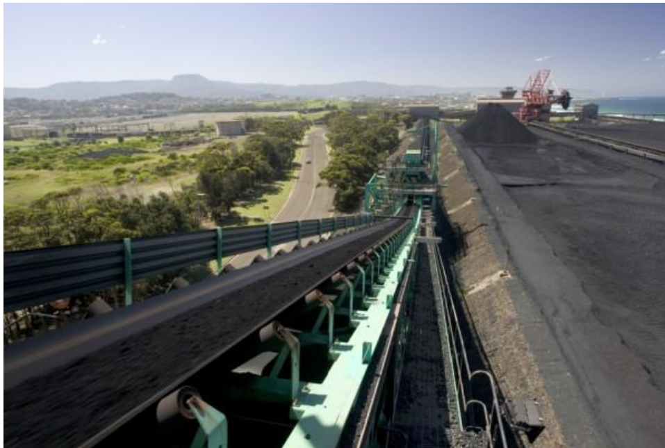
Transportation of coal via conveyor from the rail or road receive area to the stacker.
