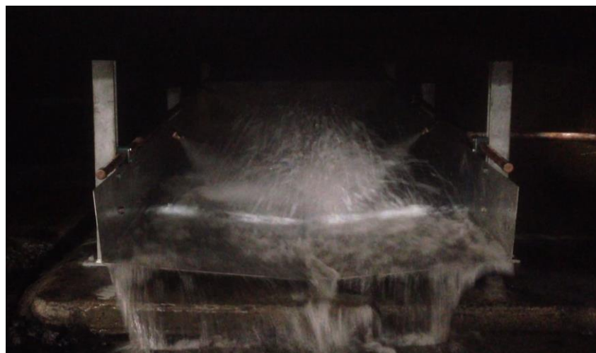
Figure 21: NC1 under-pan wash down system in action
