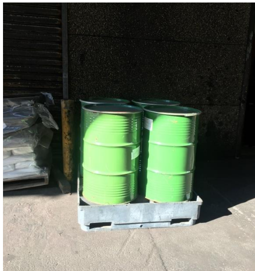
Figure 37: Contaminated waste drums on bunded pallet
