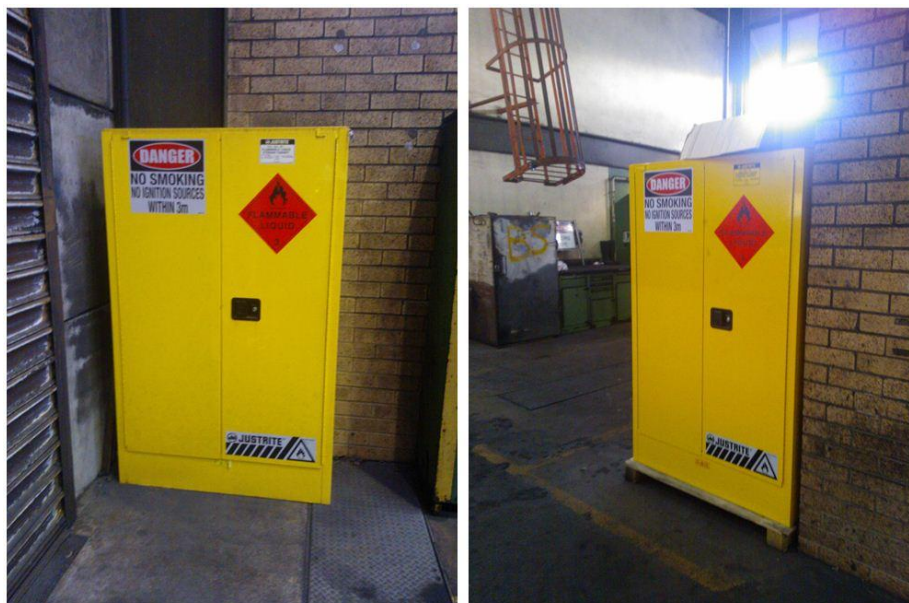
Figure 38: Two new aerosol storage cabinets introduced to East and West workshop areas.
